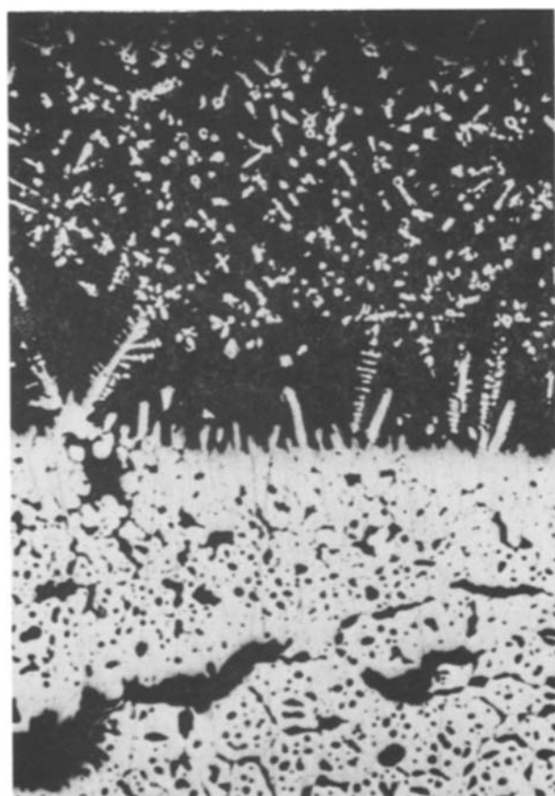
Figure 6 Cu-42% Pb space sample. Longitudinal section. Large lead accumulation in the topmost part of the sample. \times 100
